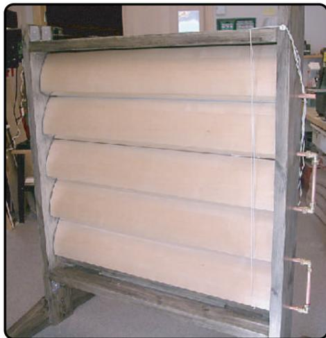
The solar wall consists of a fixed absorber with PV-cells attached to it. The heat carrying water pipes supports the components between the house's vertical wooden pillars, and are also the rotation centre for the screens, that can be turned in 90° between two modes: open and closed.
